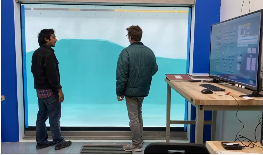
Figure 2-6: The SOARS wave tank can be used to generate rough water surface conditions with user-controlled wind and wave parameters. A transparent window in the side of the tank allows us to monitor the experimental setup and the precise height of the waves.
