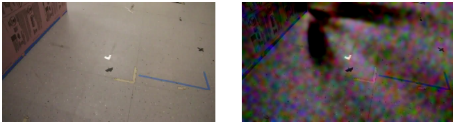
Fig. 3: Color Amplification: On the left side is an original Canon camera frame and on the right side the corresponding color-amplified frame.
