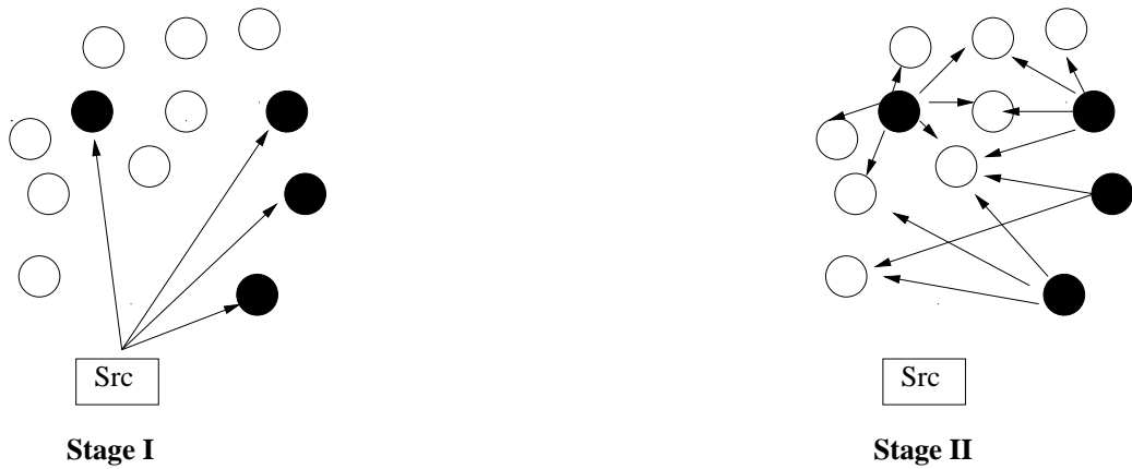
Figure 1: Illustration of the two-stage space time coded cooperative diversity scheme. In the first stage, the source node broadcasts at a high rate and only a small number of receiver nodes are able to decode. These nodes are shaded. In the second stage, these nodes cooperatively broadcast the message to the remaining nodes using a suitable space-time code protocol.
