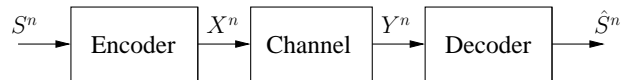
Fig. 1. Authentication system model. The source S^n is encoded to create the channel input X^n , incurring some distortion. The channel models benign degradations due to routine handling, as well as tampering by a malicious attacker. The decoder produces from the channel output Y^n either an authentic reconstruction \hat{S}^n of the source to within some fidelity, or indicates that authentication is not possible.
