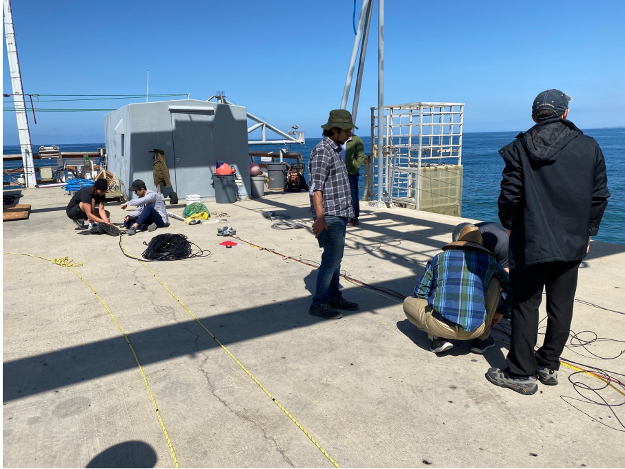
Figure 2-7: Preparing for the deployment of an emitter and a vertical receiver array at Scripps Pier. Note the weights being tied to the ends of the lines on which the emitter and receivers have been attached, intended to prevent excessive swaying in the wavy and windy ocean environment so close to the surf zone.
