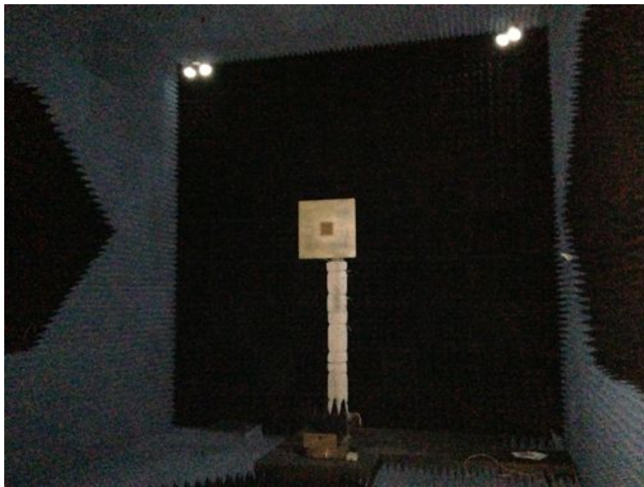
Figure 5-2: Mounted test array in anechoic antenna measurement chamber.
