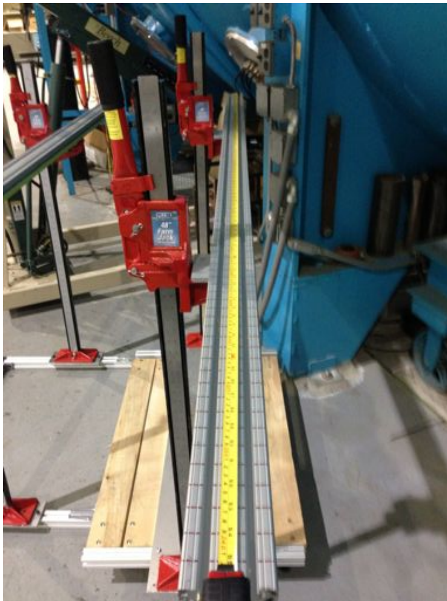
Figure 8-2: Mounting rail with markings indicating measurement locations.
