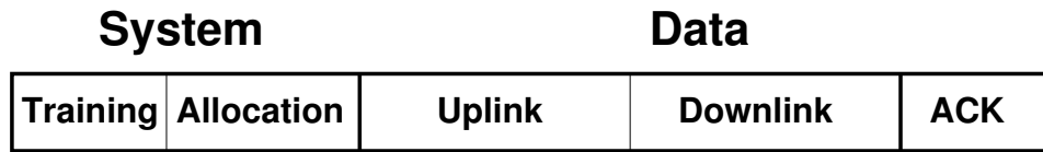
Figure 3-2: The five phases of a communications frame.
